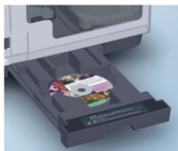
An additional drawer allows the removal of individual discs. This makes problems due to unreadable discs easy to resolve.
